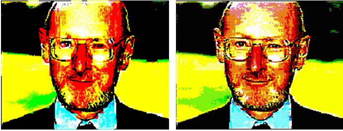
Comparison of the traditional Spectrum graphic mode (left) and the 8×1 mode of the TS 2068 (right)
