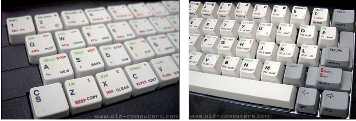
Comparison between the HC91's 40-element keyboard (left) and the 50-element one (right)
