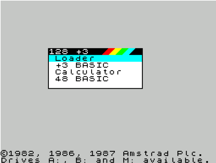
The +3's start menu. Note the indications about floppy drives A: and B: and the virtual RAM disk M:
