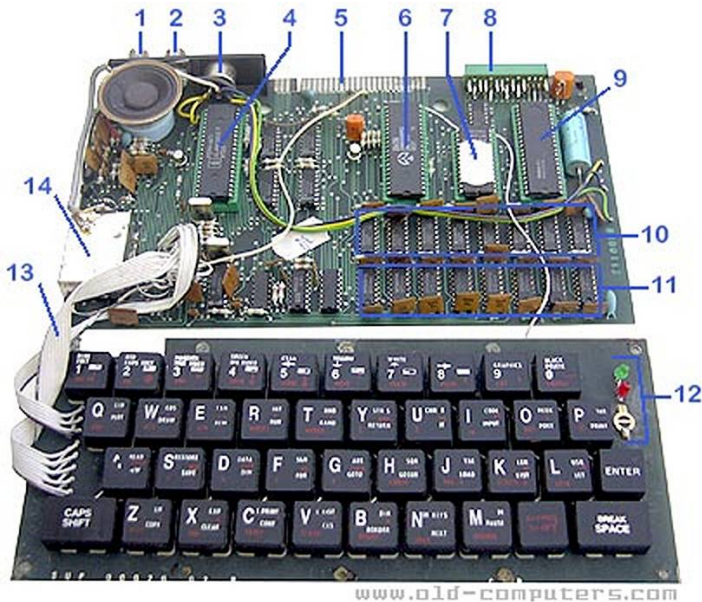
Internal view of the Didaktik Gama 87: 1-RF connector; 2-composite connector for monochrome monitors; 3-DIN input connector for the power supply unit and the tape recorder; 4-Ferranti ULA; 5- expansion port; 6- Zilog Z80A processor; 7-ROM; 8-8255 parallel port; 9-parallel port control chip; 10-Japanese-made 64 KB RAM bank; 11-Eastern European-made 16 KB RAM banks; 12-power LED (green), bank-switching activation LED (red) and reset button; 13-keyboard cable soldered on both sides, which makes it impossible to detach the keyboard from the motherboard; 14-RF TV modulator.
