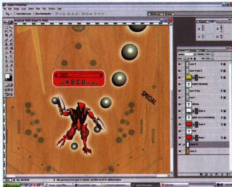
FIGURE 13: In your paint software, layer up the decals over the wooden texture using the exported blueprint as a guide.
